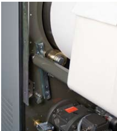
Kinematic strap tensioning system (Pat 0528745) that ensures optimum ironing quality.
