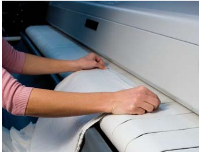
Hand guard protection with double sensor to control the active and rest position.
